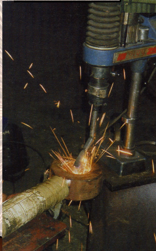
Automated ID (bore) welder, welding an eye before machining takes place.
